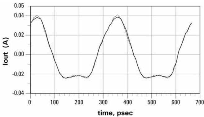
Fig. 5. Time-dependent output waveform validation. Behavioral Model (dotted), Independent large-signal measurements (solid).
