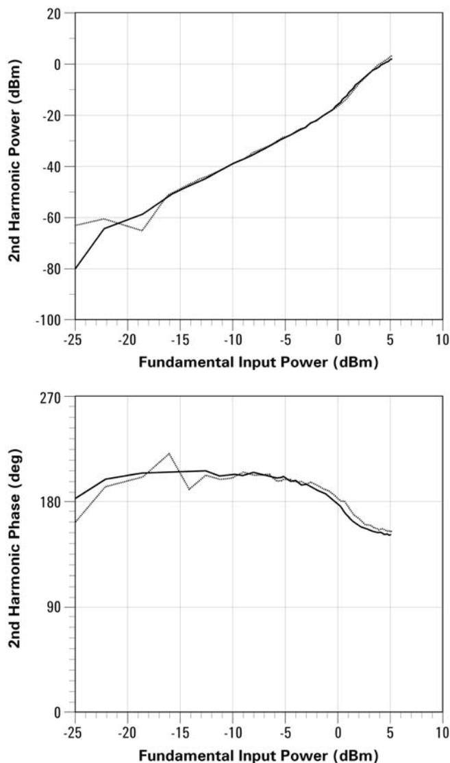
Fig. 3. Second harmonic amplitude (top) and phase (bottom). Behavioral Model (dotted) and load-pull data (solid).
