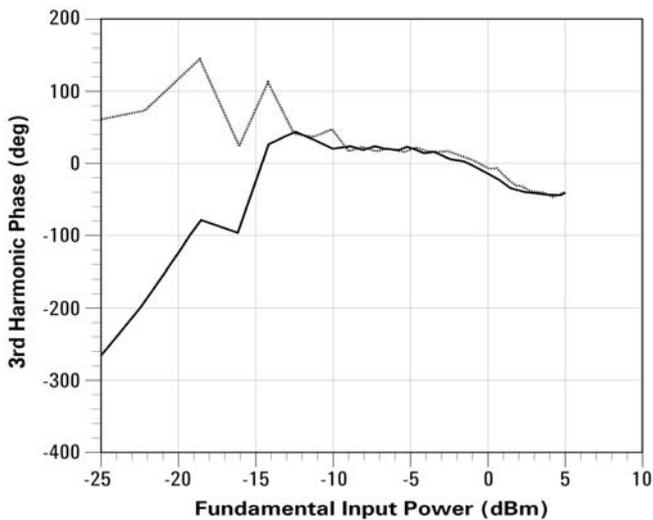
Fig. 4 Third harmonic amplitude (top) and phase (bottom). Behavioral Model (dotted) and load-pull data (solid)
