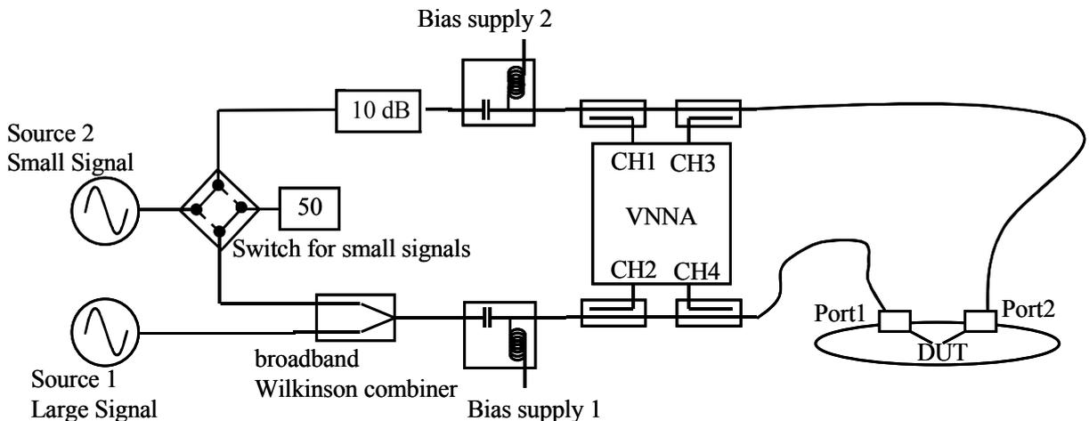
Fig. 1. Schematic connection of the VNNA for the large-signal and small-signal perturbations to the DUT
