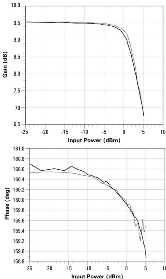
Fig. 2. Fundamental Gain compression (AM-AM) (top) and phase variation (AM-PM) (bottom) as a function of input power. Behavioral Model (dotted) and load-pull validation (solid).
